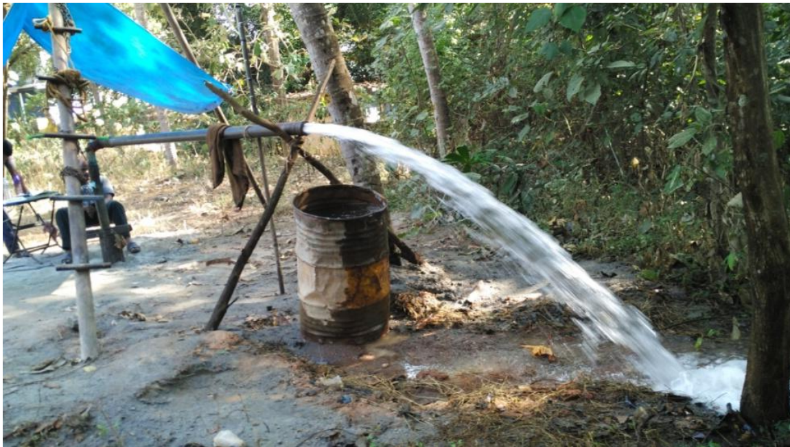
Fig 3.3 . Pumping test at Cherpulassery Exploratory well (discharge 16.00 Lps), Kerala
